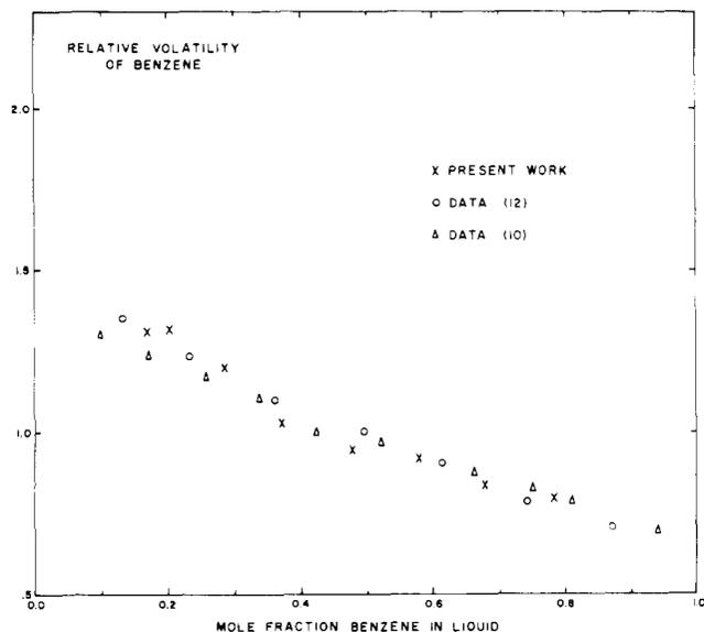
Figure 3. Relative volatility-composition diagram for benzene-cyclohexane at 40 °C
