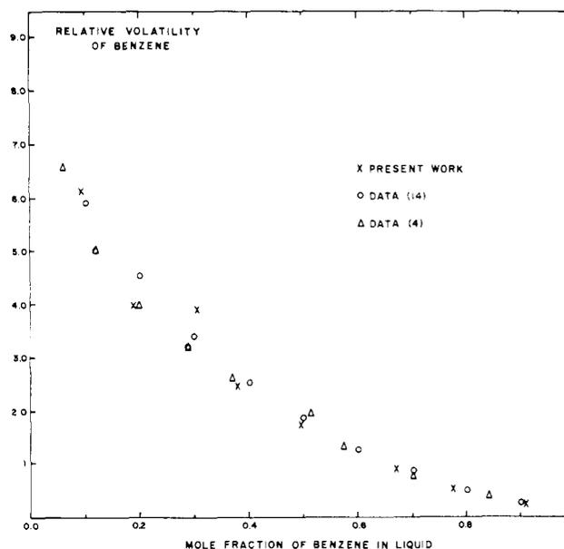
Figure 5. Relative volatility-composition diagram for benzene-ethyl alcohol system at 25 °C
