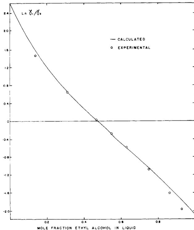
Figure 8. Redlich-Kister plot for ethyl alcohol-*n*-heptane system at 30 °C
