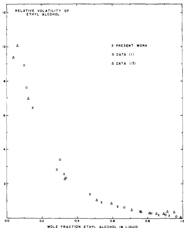
Figure 4. Relative volatility-composition diagram for ethyl alcohol-n-heptane system at 30 °C
