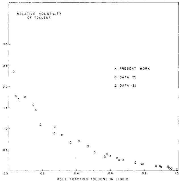
Figure 6. Relative volatility-composition diagram for toluene-ethyl alcohol system at 35 °C
