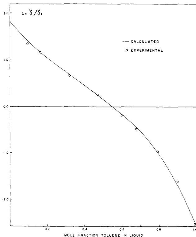
Figure 10. Redlich-Kister plot for toluene-ethyl alcohol system at 35 °C
