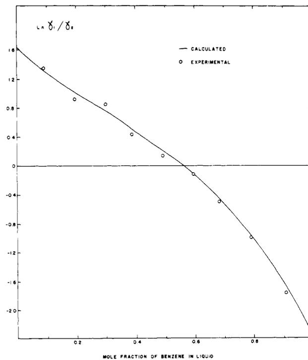
Figure 9. Redlich-Kister plot for benzene-ethyl alcohol system at 25 °C
