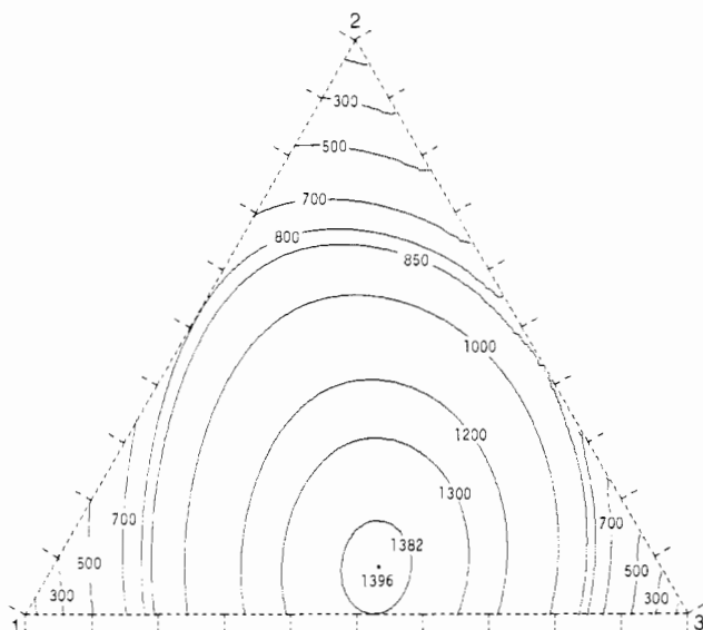
Figure 3. Computer-generated contour diagram showing lines of constant G^E_{123} (in J/mol) on a liquid-mole-fraction grid for acetonitrile (1)-ethanol (2)-water (3) at 50 °C.
