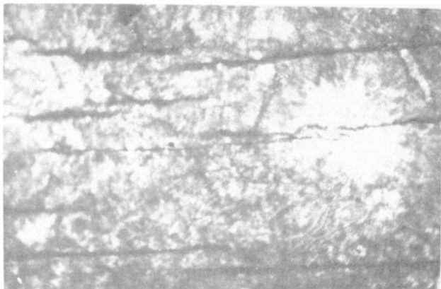
Figure 9. Microphotograph of directionally solidified picric acid-cinnamic acid eutectic containing 0.6600 mole fraction of picric acid \times 100 .
