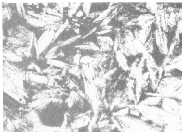
Figure 11. Microphotograph of directionally solidified picric acid-cinnamic acid 1:1 addition compound \times 100 .
