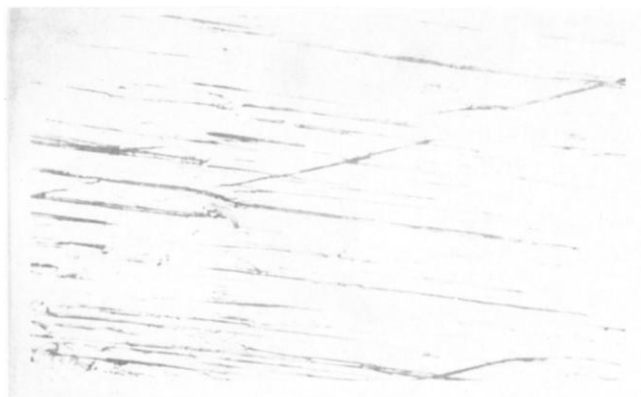
Figure 7. Microphotograph of directionally solidified picric acid \times 100 .
