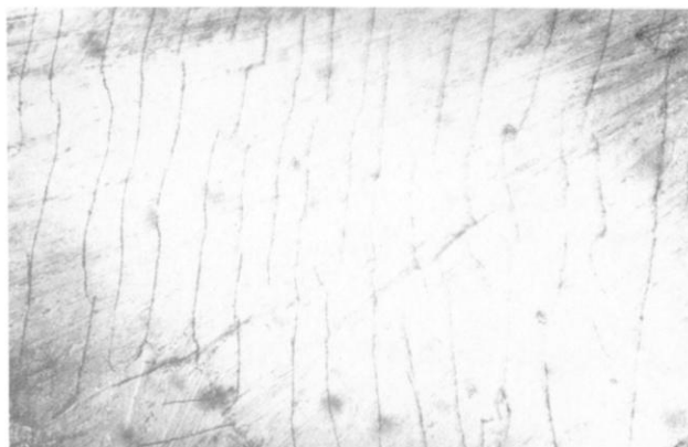
Figure 10. Microphotograph of directionally solidified picric acid-cinnamic acid eutectic containing 0.4200 mole fraction of picric acid \times 100 .
