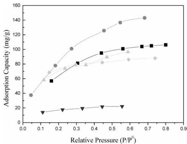
**Figure 3.** Adsorption capacities for aromatics adsorbed by silica gel at different pressures: ■, benzene; ●, toluene; ▲, *o*-xylene; ▼, *p*-xylene; ◆, *m*-xylene.
