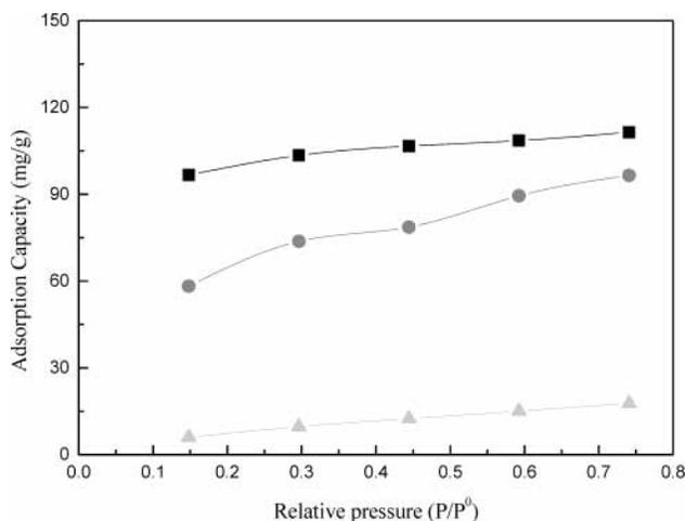
**Figure 6.** Adsorption capacities for *o*-xylene adsorbed by different sorbents at different pressures: ■, activated carbon; ●, silica gel; ▲, 13X zeolite.
