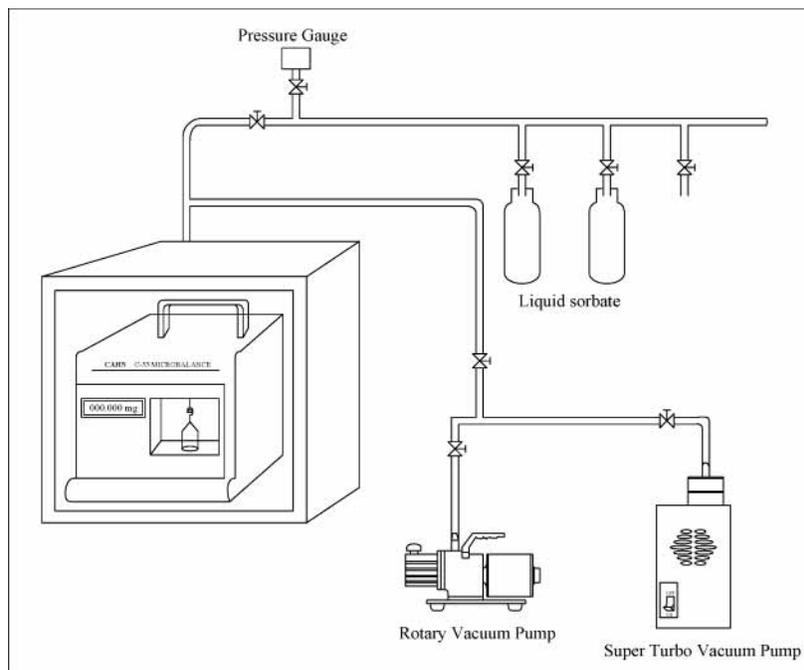
**Figure 1.** The gravimetric adsorption apparatus of this study (static gravimetric method).
