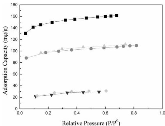
**Figure 2.** Adsorption capacities for aromatics adsorbed by activated carbon at different pressures: ■, benzene; ●, toluene; ▲, *o*-xylene; ▼, *p*-xylene; ◆, *m*-xylene.
