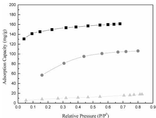
**Figure 5.** Adsorption capacities for benzene adsorbed by different sorbents at different pressures: ■, activated carbon; ●, silica gel; ▲, 13X zeolite.
