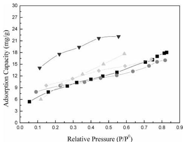
**Figure 4.** Adsorption capacities for aromatics adsorbed by 13X zeolite at different pressures: ■, benzene; ●, toluene; ▲, *o*-xylene; ▼, *p*-xylene; ◆, *m*-xylene.
