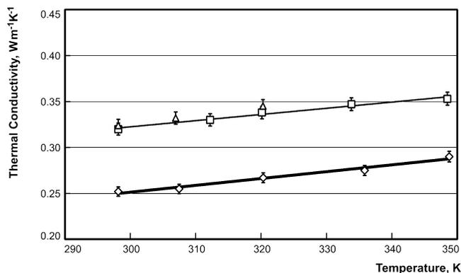
**Figure 7.** Thermal conductivity  $\lambda$  measurements as a function of temperature  $T$ :  $\diamond$ , epoxy-resin polymer measurements; —, eq 1;  $\square$ , epoxy-resin polymer + glass fiber measurements; —, eq 2;  $\Delta$ , epoxy-resin polymer + glass fiber (samples cut at 60° angle from principal axis) measurements.
