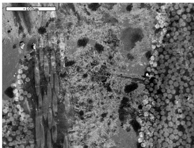
Figure 4. SEM image of samples with C-MWNT mass fraction of 0.25 %.
