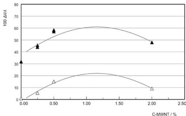
**Figure 8.** Enhancement of the thermal conductivity measurements,  $100 \Delta\lambda/\lambda$ , as a function of the composition of the C-MWNT mass fraction:  $\Delta$ , epoxy resin + C-MWNT;  $\blacktriangle$ , epoxy resin + C-MWNT + glass fibers. Black lines show trends only.
