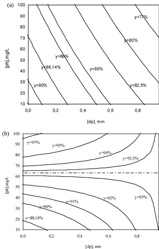
**Figure 6.** Iso-response plots in the plane initial concentration of phenol/ particles size for (a)  $[Ac] = 1 \text{ g}\cdot\text{L}^{-1}$ , (b)  $[Ac] = 2 \text{ g}\cdot\text{L}^{-1}$ .
