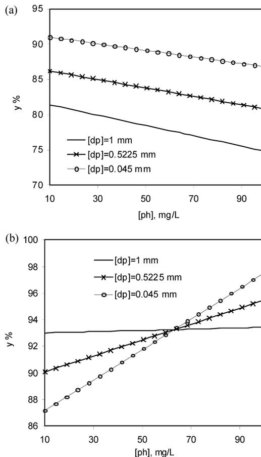
**Figure 7.** Evolution of the amount of adsorption versus initial concentration of phenol. (a)  $[Ac] = 1 \text{ g}\cdot\text{L}^{-1}$ ; (b)  $[Ac] = 2 \text{ g}\cdot\text{L}^{-1}$ .
