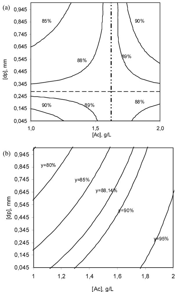
**Figure 4.** Iso-response plots in the plane particle size versus concentration of suspension. (a)  $[\text{ph}] = 10 \text{ mg} \cdot \text{L}^{-1}$ ; (b)  $[\text{ph}] = 100 \text{ mg} \cdot \text{L}^{-1}$ .
