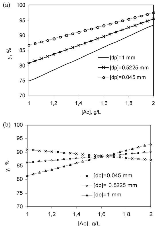
**Figure 9.** Evolution of the amount of adsorption versus concentration of activated carbon. (a)  $[ph] = 100 \text{ mg}\cdot\text{L}^{-1}$ ; (b)  $[ph] = 10 \text{ mg}\cdot\text{L}^{-1}$ .
