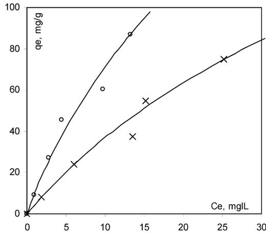
**Figure 3.** Phenol isotherms on activated carbon ( $2 \text{ g} \cdot \text{L}^{-1}$ ) for two particle diameter:  $\circ$ , powder;  $\times$ , granular (comparison with the model (full lines)).
