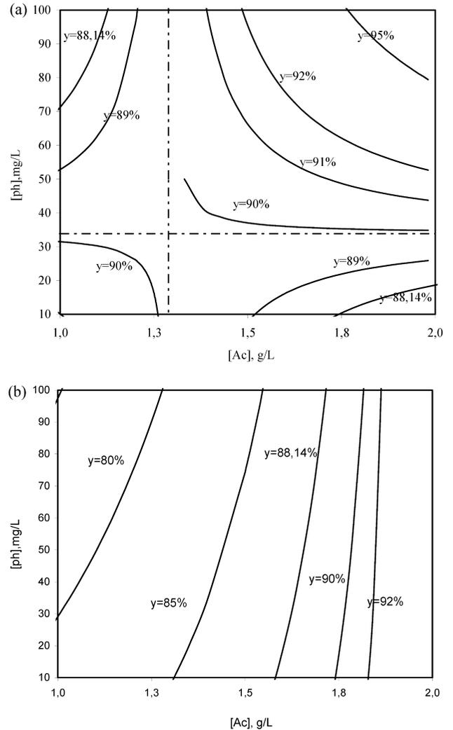
**Figure 5.** Iso-response plots in the plane initial phenol concentration/concentration of suspension. (a)  $[\text{dp}] = 1 \text{ mm}$ ; (b)  $[\text{dp}] = 0.045 \text{ mm}$ .
