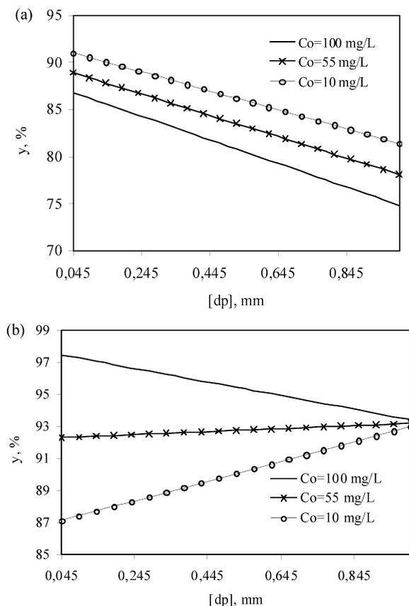
**Figure 8.** Evolution of the amount of adsorption versus particle diameter. (a)  $[Ac] = 1 \text{ g}\cdot\text{L}^{-1}$ ; (b)  $[Ac] = 2 \text{ g}\cdot\text{L}^{-1}$ .
