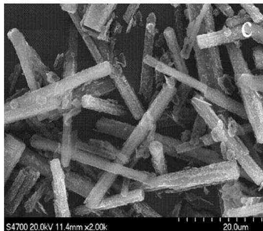
**Figure 12.** SEM images of MgCO<sub>3</sub>·3H<sub>2</sub>O in mixed solutions (LiCl + MgCl<sub>2</sub>) at 308 K after 6 h.
