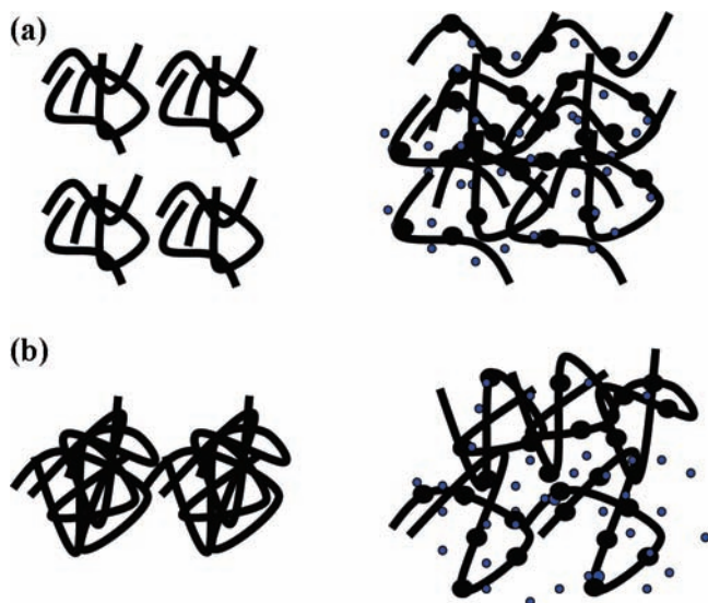
Figure 5. Schematic drawing of the interactions in the PAA/Na 2 CO 3 /water system: (a) small chains and (b) large chains. The black disks on the chain backbone represent the globular structure, while the blue disks surrounding the backbone represent the ionic species of salt.
