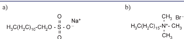
Figure 2. Molecular formula of the surfactants: (a) SDS and (b) HDTA.
