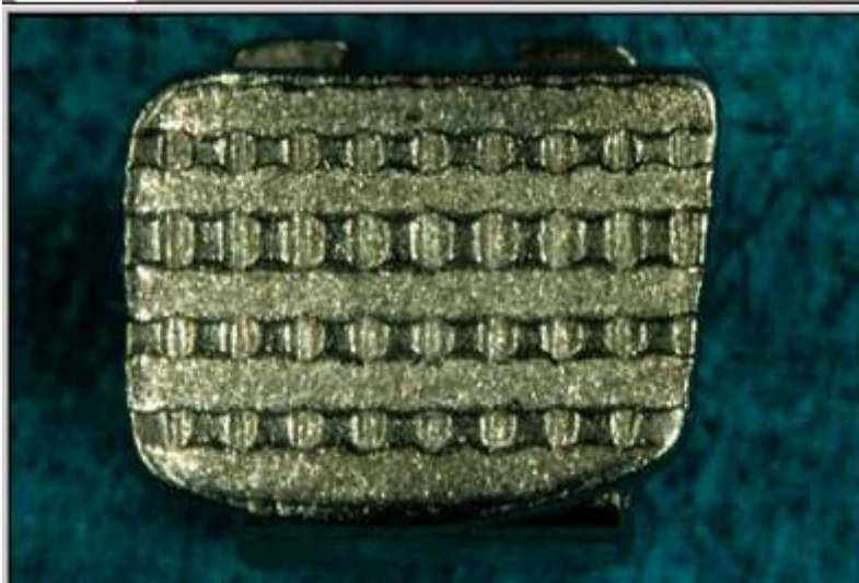
Fig. 7 Microetched mechanical undercuts on Time bracket base.
