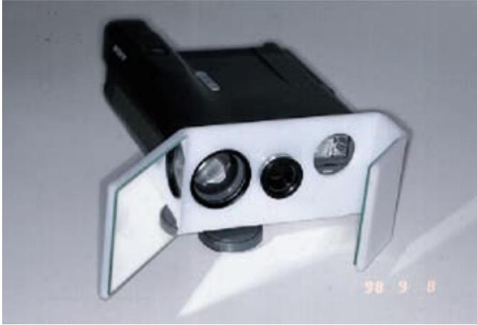
Fig. 5 Light deflector on digital camera corrects asymmetry of flash unit.
