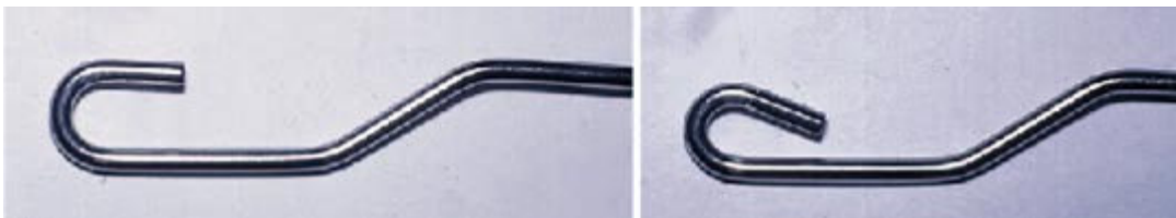
Fig. 4 End of outer bow bent inward to prevent laceration injuries.
