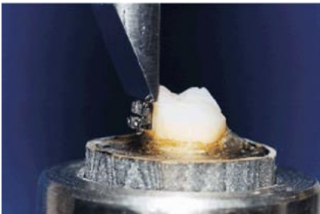
Fig. 2 Shear force applied to bracket in Instron machine.
