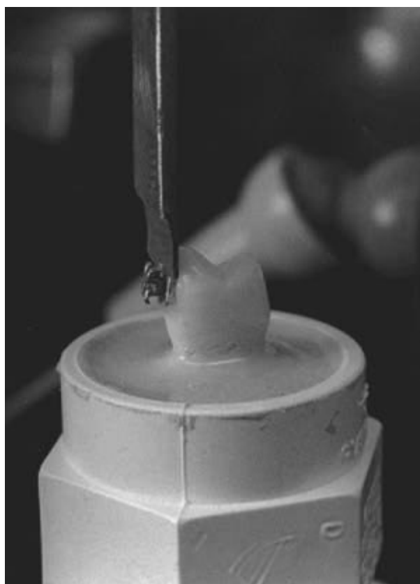
Fig. 1 Shear bond strength testing apparatus.
