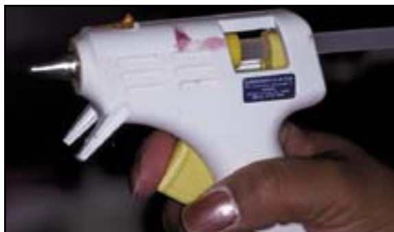
Fig. 1 Surebonder DT-200 dual-temperature hot-glue gun.
