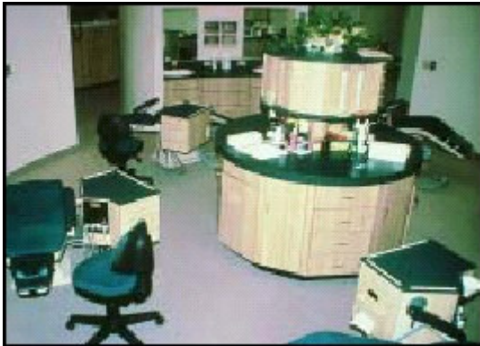
Fig. 7 Four-chair corner arrangement, requiring 475 square feet
