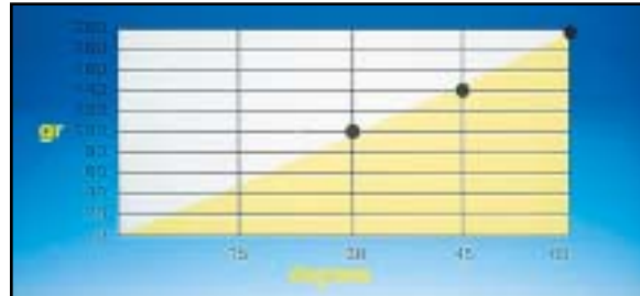
Fig. 2 Forces in grams delivered at 30°, 45°, and 60° of activation (adapted from Hilgers 5 ).
