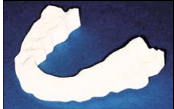
Fig. 8 Occlusal splint photopolymerized by laser lithography unit.
