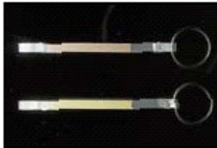
Fig. 4 Oscillating Elastrips, fine (top) and ultrafine (bottom), used for polishing.
