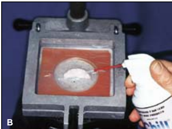
Fig. 3 A. Tray plastic thermoformed over cast and rubber band. B. Hot plastic sprayed with refrigerant immediately after thermoforming.
