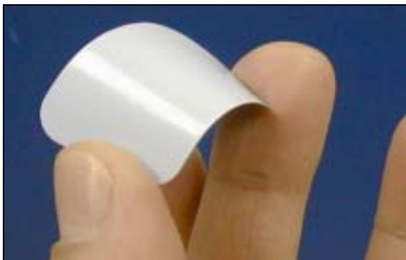
Fig. 1 Storage phosphor imaging plates are thin and flexible like conventional film; unlike CCD sensors, they do not have to be connected to computer by wire.
