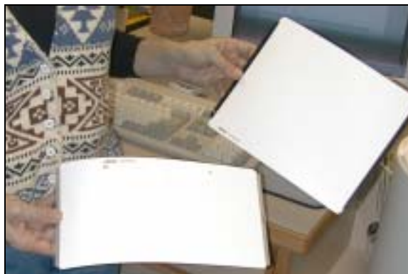
Fig. 3 Panoramic and cephalometric imaging plates require only removal of lanex screen from film cassette of any pan/ceph machine.
