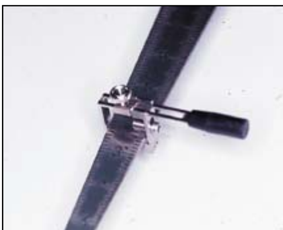
Fig. 5 In-out control of bracket positioning by measuring labiolingual width of widest tooth with special millimeter ruler and fixing in-out stopper. Jigs of all anterior teeth are then slid same distance.
