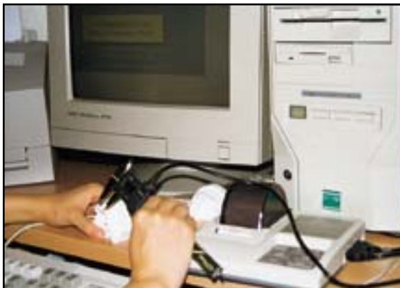
Fig. 2 Digital calipers connected to computer via Mitutoyo Digimatic Mini Processor.
