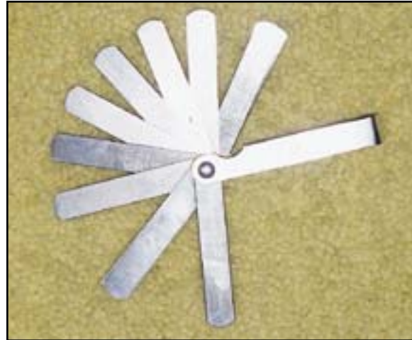
Fig. 3 Common sparkplug-gap leaf gauge (#36A**).
