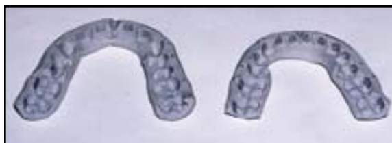
Fig. 10 Index mark cut in each tray to indicate midlines.
