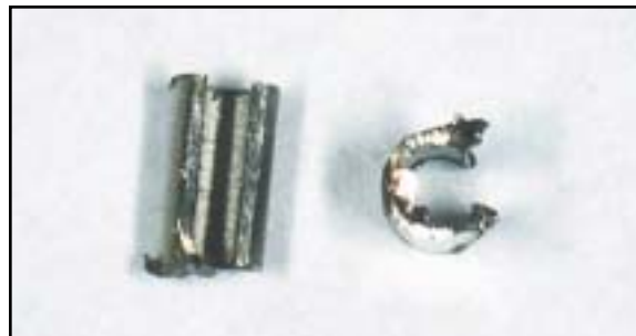
Fig. 3 Two views of stainless steel split tubing used for reactivation.
