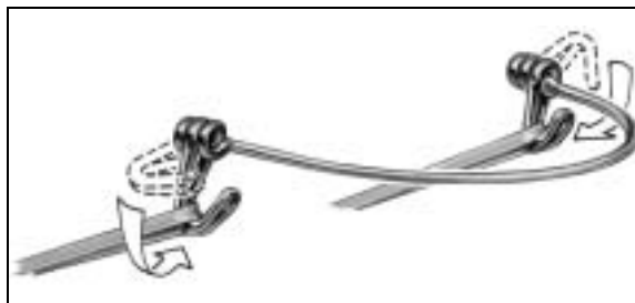
Fig. 1 Outrigger has coiled ends with hooks for Class II elastic engagement.
