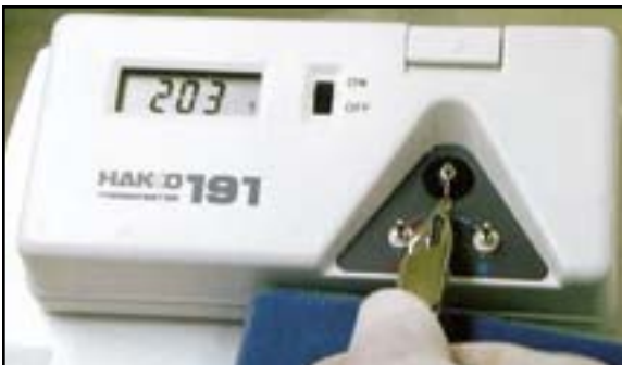
Fig. 5 Hakko digital thermometer used to verify wedge temperature.
