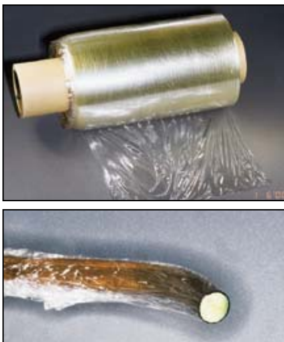
Fig. 4 Reynolds Perforated 920 Cling Film is supplied in roll of 6" × 5" perforated sheets of polyvinyl chloride (PVC).
