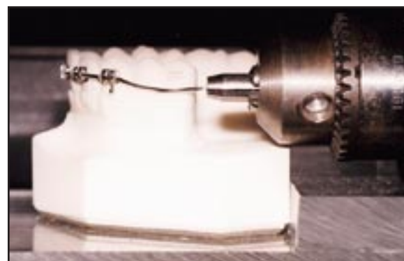
Fig. 3 Wire twisted 180° and tied into brackets.
