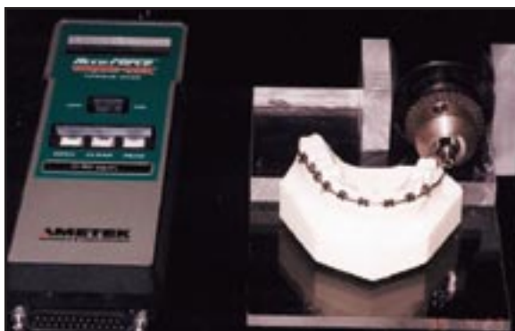
Fig. 1 Torque-measuring apparatus: torque gauge, typodont, acrylic base.
