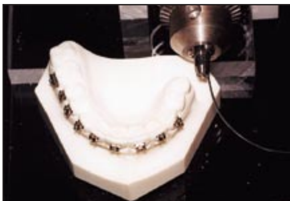
Fig. 2 Wire inserted into clamp of torque gauge, simulating molar tube.
