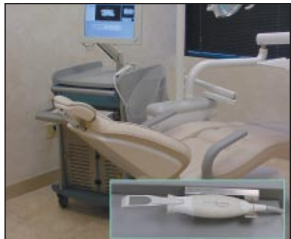
Fig. 3 OraScanner and computer housed in chair-side SureSmile cart.
