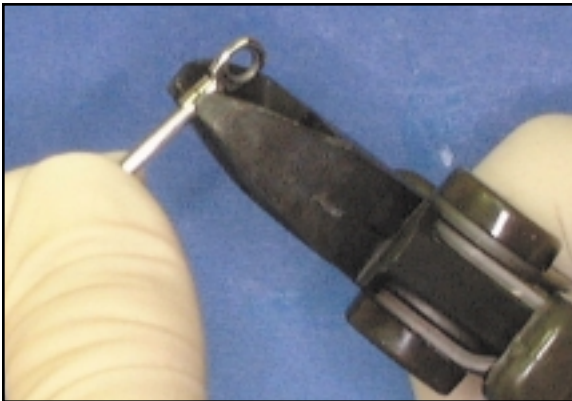
Fig. 4 Shim crimped in place with heavy wire cutter.
