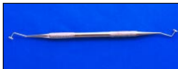
Fig. 2 Needle tubes soldered at right angles to excavator tips.
