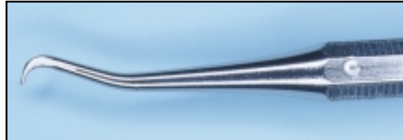
Fig. 2 Ideal opening instrument has slender, rigid tip, just long enough to seat against internal guide slot when fully inserted.
