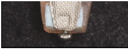
Fig. 3 For rebonding, new bracket fits securely into original hybrid core.
