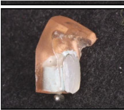
Fig. 1 Hybrid core consists of resin part (red) and silicone part (green).
