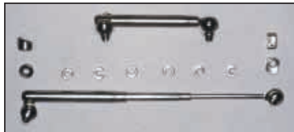
Fig. 5 HTH components, showing split crimpable shims used for reactivation.
