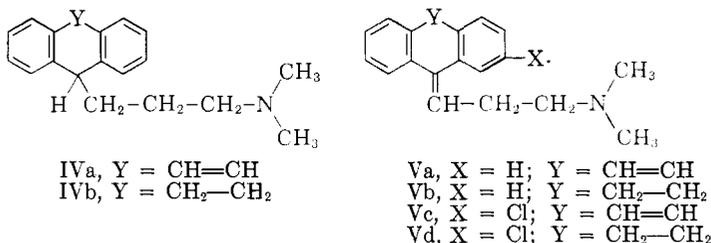
The synthetic approach to IVa involved the alkylation of the potassium derivative of 5H-dibenzo[a,d]cycloheptene (VI) with  $\gamma$ -dimethylaminopropyl chloride.<sup>5</sup> Compound IVa was isolated in a yield of 57% and the method was extended to the alkylation of VI with  $\beta$ -dimethylaminoethyl chloride and 1-(3-chloropropyl)-4-methylpiperazine to give the desired compounds in 46% and 12% yields respectively.
