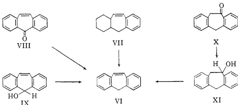
by reduction with zinc and ammonium hydroxide and by lithium aluminum hydride. This compound was treated with thionyl chloride and the resulting chloride was reduced with zinc and acetic acid to give VI in 40–45% yield. Alternatively, carbinol IX was reduced to VI with phosphorus and iodine in very poor yield.
