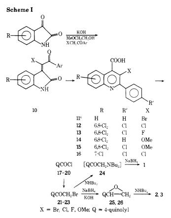
ketone 21 with NHBu<sub>2</sub> and NaBH<sub>4</sub> reduction to 1, and NaBH<sub>4</sub>-KOH reductions of bromo ketones 22 and 23 to epoxides 25 and 26 followed by condensations with NHBu<sub>2</sub> to 2 and 3.
