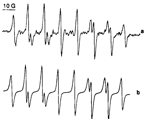
Figure 2. (A) ESR spectrum of DEPMPO-OOH obtained as a consequence of the reaction of hypoxanthine with xanthine oxidase. Spectrometer settings were microwave power, 10 mW; modulation frequency, 100 kHz; modulation amplitude, 1 G; receiver gain 6.3 \times 10^3 ; response time 0.128 s; sweep time 52.5 G/min. (b) Computer simulation of (a) obtained with the parameters listed in Table 1.
