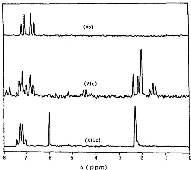
Fig. 1. <sup>1</sup>H NMR spectra of  $[(p\text{-ClC}_6\text{H}_4\text{C})_4\text{PdBr}_2]_2$ , (Vb);  $[\text{endo-EtO}(p\text{-CH}_3\text{C}_6\text{H}_4)_4\text{C}_4\text{PdCl}]_2$ , (VIc) and  $[(p\text{-CH}_3\text{C}_6\text{H}_4)_4\text{C}_4\text{PdC}_5\text{H}_5]\text{Br}$  (XIIc) in CDCl<sub>3</sub>.
