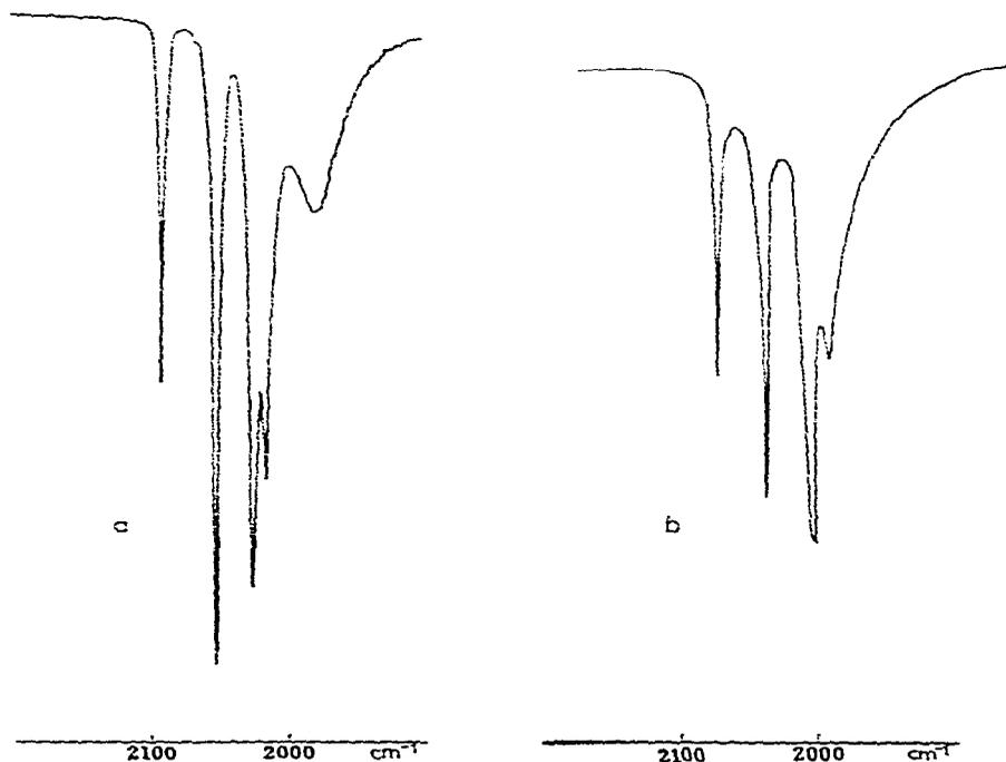
Fig. 1. Infrared spectra in carbon tetrachloride in the 2100-2000  $cm^{-1}$  region of: (a),  $C_4H_4Fe_2(CO)_5$ ; (b),  $(C_6H_5)_3C_4Fe_2(CO)_5$ .
