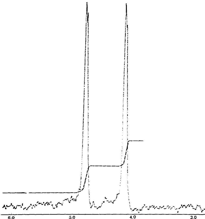
Fig. 2. NMR spectrum of  $C_2H_2Fe_2(CO)_5$  in carbon tetrachloride. Chemical shifts are recorded in ppm downfield from tetramethylsilane.
