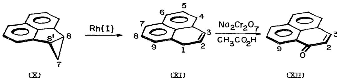
$^1\text{H}$  NMR spectroscopy since the characteristic aliphatic proton signals of X [17] and those due to H(1)—H(3) in XI [18] are widely separated. Additional confirmation of structure was achieved through oxidation of XI with sodium dichromate in acetic acid [16] to give phenalenone (XII) whose identity was established by spectral means [18] and direct comparison with a commercial sample.
