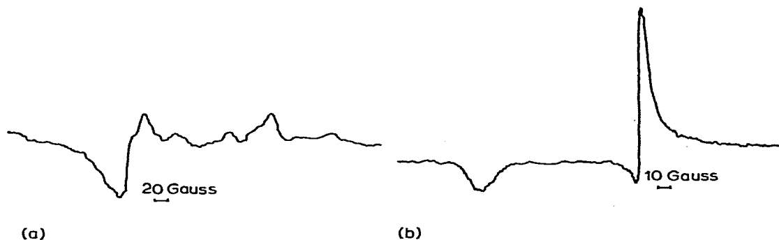
Fig.1. (a) EPR spectrum of C_6H_5FeC_5H_5 at 14 K, (b) EPR spectrum of C_{10}H_8FeC_5H_5 at 77 K.
