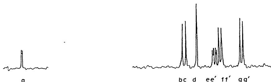
Fig. 3. ^{13}\text{C} NMR low-temperature limiting spectrum of \text{HRu}_3(\text{CO})_{10}(\text{COCH}_3) at -100^\circ\text{C} (proton-coupled).
