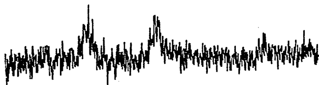
Fig. 2. ^{125}\text{Te} NMR spectra of an equilibrium mixture of \text{C}_8\text{H}_8\text{TeCl}_2 and \text{C}_8\text{H}_8\text{TeBrCl} in \text{DMF-}d_7 . 10,000 transients; 3.6 sec delay; proton noise decoupling.
