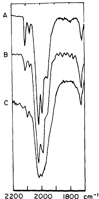
Fig. 5. Infrared spectra of (A) synthetic mixture of \text{PPN}[\text{HRu}_3(\text{CO})_{11}] and \text{PPN}[\text{Ru}(\text{CO})_3\text{I}_3] (2/1 molar ratio), (B) catalytic mixture obtained from \text{Ru}_3(\text{CO})_{12} and KI in sulfolane, after catalysis, and (C) same catalytic mixture during catalysis at 55.1 MPa \text{H}_2/\text{CO} , 230°C.
