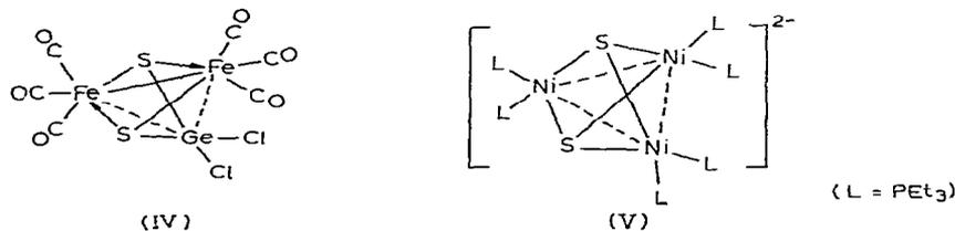
The distances between the M atoms in the trigonal bipyramidal skeleton may, depending on the nature of M and other ligands, vary from purely non-bonded (average Ni—Ni distance in V is 2.91 Å) to short M—M bonds (two Fe—Fe bonds of 2.59 Å (average) in  $\text{Fe}_3(\text{CO})_9\text{S}_2$ , mentioned above, and the Fe—Fe bond of 2.480 Å in IV).
