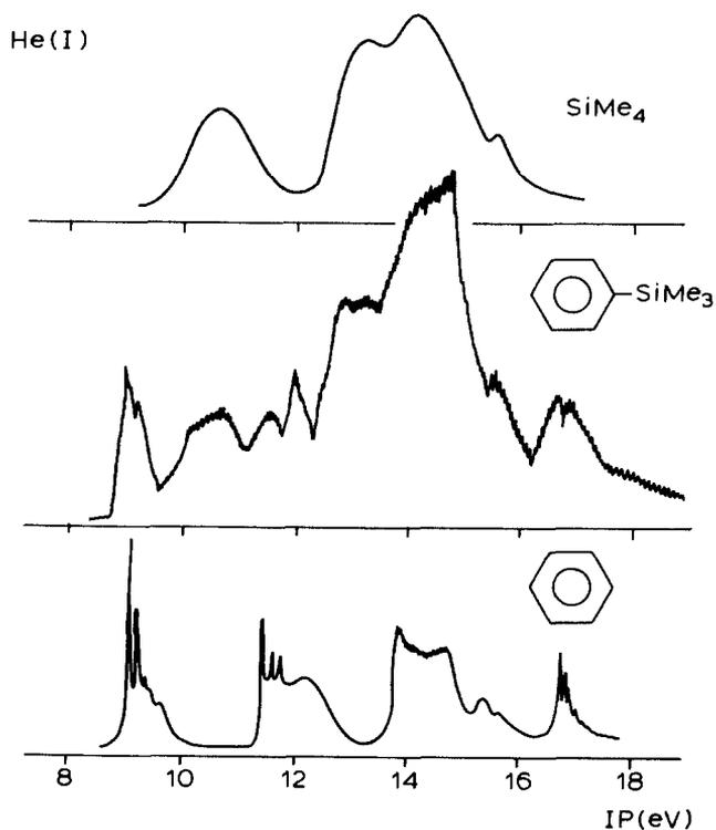
Fig. 1. He(I) photoelectron spectrum of benzene, trimethylphenylsilane and tetramethylsilane.
