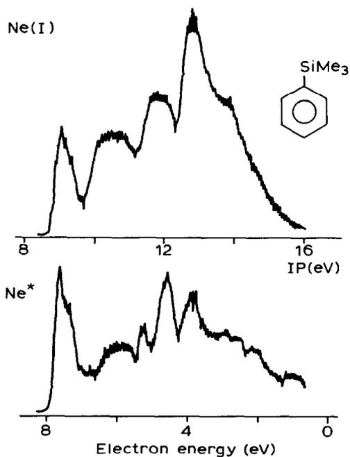
Fig. 2. Ne(I) UPS and Ne\* PIES of trimethylphenylsilane.
