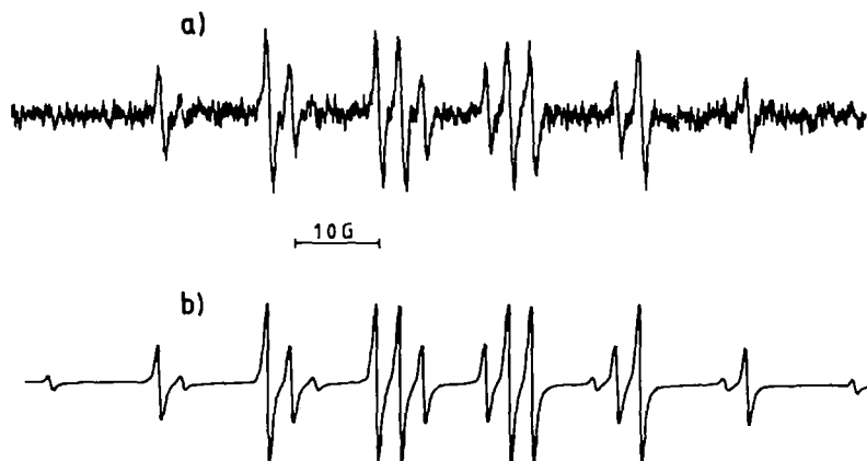
Fig. 1. (a) ESR spectrum of methyl(trimethylsilylmethyl)amine- N -oxyl (1c) in benzene at room temperature; (b) simulated spectrum.
