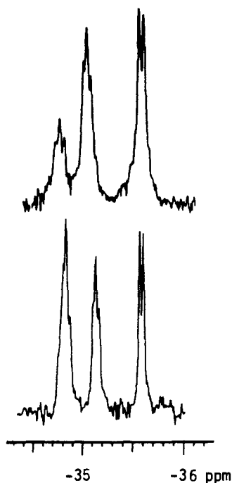
Fig. 2. ^{29}\text{Si} \{^1\text{H}\} NMR of the \text{D}^{\text{H}} region of \text{MD}_5^{\text{H}}\text{M} (upper) and \text{MD}_7^{\text{H}}\text{M} (lower) oligomers.
